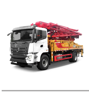
Boom Pump (Concrete)
