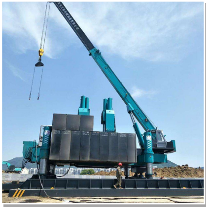
PHC Pile Hammer
